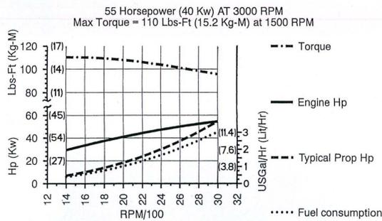
Westerbeke recommends a propeller that will allow the engine to turn 3000 RPM underway at full throttle
